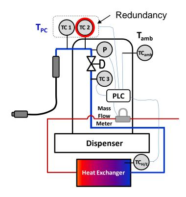
Because the fuel delivery temperature is directly used to calculate the pressure ramp rate, it should have a high reliability, i.e. redundant sensors.
