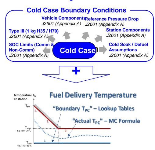
• In addition to the hot and cold case boundary conditions, the fuel delivery temperature also is used to determine the Pressure Ramp Rate and End-of-Fill Pressure Target
