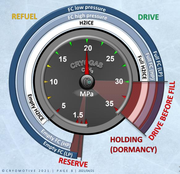
• Usable range depends on the minimum supply pressure between 0.6 MPa and 5 MPa to 30 MPa
