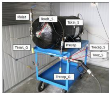
Figure 3 - Model validation [5] for protocol development for light duty vehicles in [2]
